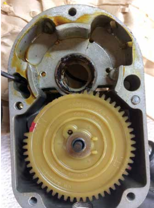
Photo 1: The failed magneto clearly missing about 25% of its drive-gear teeth. Yet, enough teeth remained to allow it to function in a reduced and intermittent capacity (which was probably worse than if it had just totally failed).
