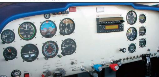
a multi-phased panel makeover (see sidebar). Upon certification, the Aspen MFD was able to act as the backup airspeed indicator and altimeter, but the FAA demanded that the backup attitude information come from a completely separate source. To address this complication, a Mid-Continent 4300-Series LifeSaver® electrical attitude indicator was installed.
