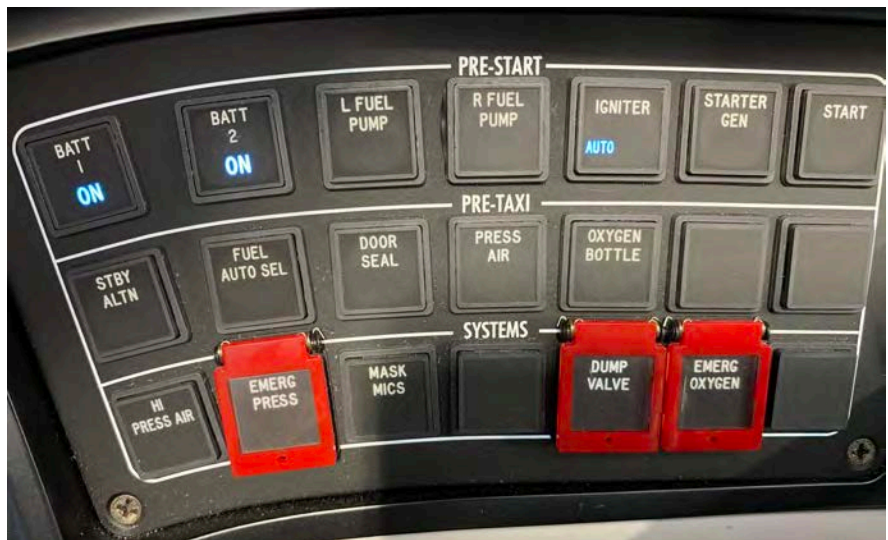
One example of the design of the various E1000 GX's subpanels, organized into logical rows and groups with sequential button placement to create easy workflows.
