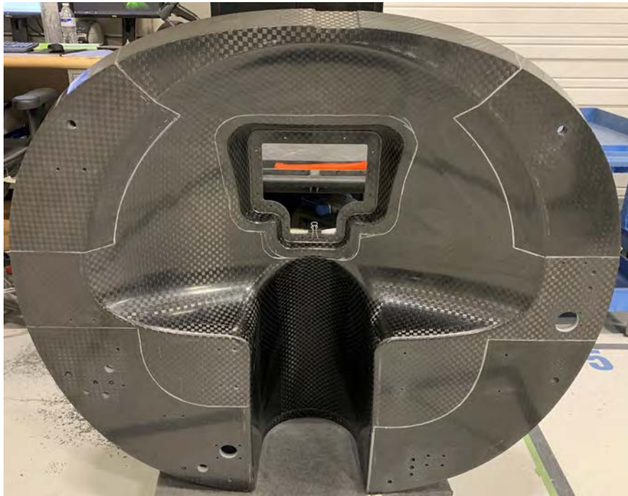
The primary carbon-fiber construction material makes up all major structures, all flight controls, trim tabs, cabin panels and flooring, most fairings and trim pieces, and even the firewall (shown here).
