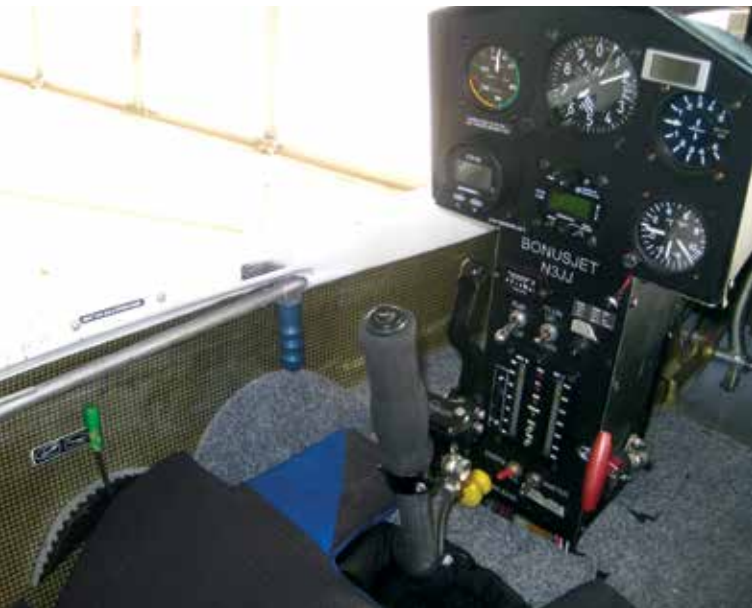
The TST-14J BonusJet panel. The lower console is dedicated to the PBS engine gauges and extension/retraction control. On the upper panel, the fuel gauge and voltmeter were exchanged for units appropriate to the jet engine. The left sidewall houses the thrust lever (black), trim lever (green), and spoiler lever (blue). The hand brake lever on the control stick activates the powerful Berringer disc brake on the main landing gear.
