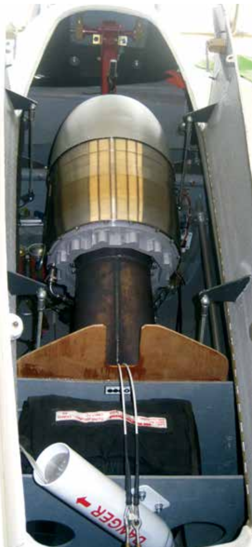
The fully encloseable engine bay of the BonusJet motor glider houses both the retracted PBS TJ-100 engine (forward) and the BRS ballistic parachute recovery system (aft).
