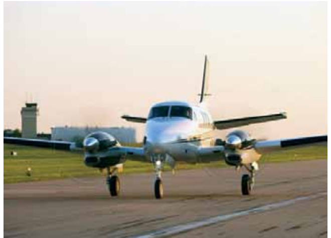
To help save fuel while taxiing, apply just enough power to get the aircraft rolling, while using minimum power and braking. Utilizing Beta thrust can be very effective in controlling taxi speed, lessening the need for braking.
