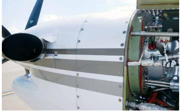
A close-up of the modification Blackhawk designed and manufactured to extend the internal air intake seal far enough aft to fully encase the air intake section of the longer -67A engine.
