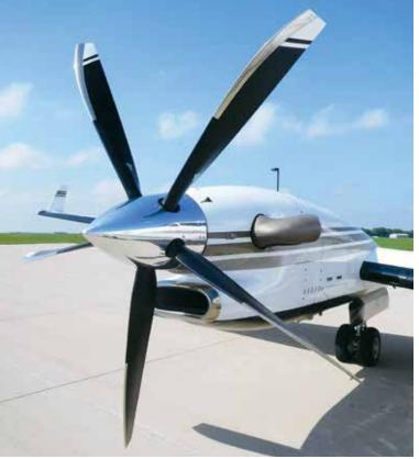
The 5-bladed, composite MT propellers perform as good as they look. They offer a number of advantages over the stock, 4-blade metal props, not the least of which is offsetting the weight penalty of the heavier -67A engines.
