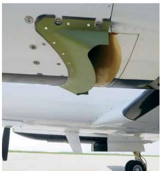
A closer look at the new fixed flap and modified oil cooler air exit port, which helps improve oil cooling, allowing higher ITT limits.
