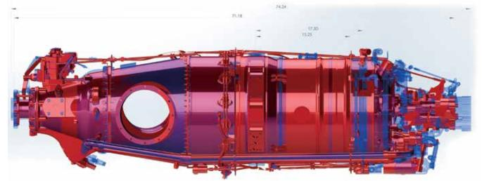
An overlay of the PT6A-60A (red) and the -67A (blue) engines shows the extra length of the -67A that needed to be wedged into the same cowling as the original -60As. (COURTESY BLACKHAWK)
