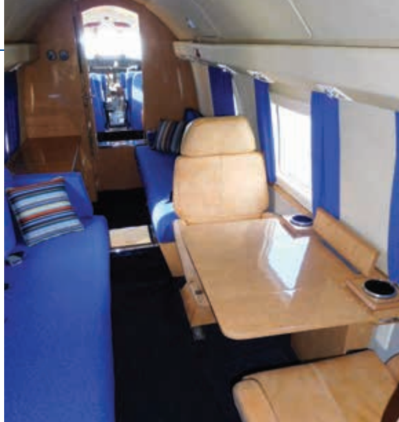
The stand-up cabin of N500LN accommodates 12 passengers in executive-level comfort. Each set of club seats in an executive-configured Howard 500 cabin included a stowable work table and cup holders to complement the adjustable leather seats.
