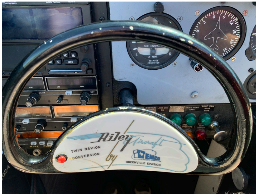
The pilot-side yoke of the Twin Navion. TEMCO produced the aircraft for Riley in Texas after Riley's facility in Florida could not meet demand. Initially, as the Twin-Riley (D-16), then as the Riley-55 (D-16A).
