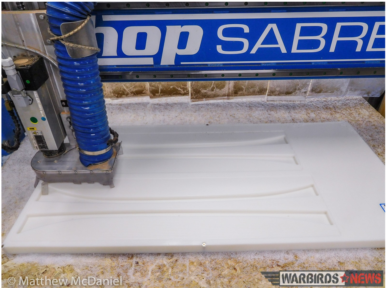
Precise molds being cut by computer controlled machinery for the future fabrication of new Helldiver wing ribs. (photo by Matthew McDaniel)
