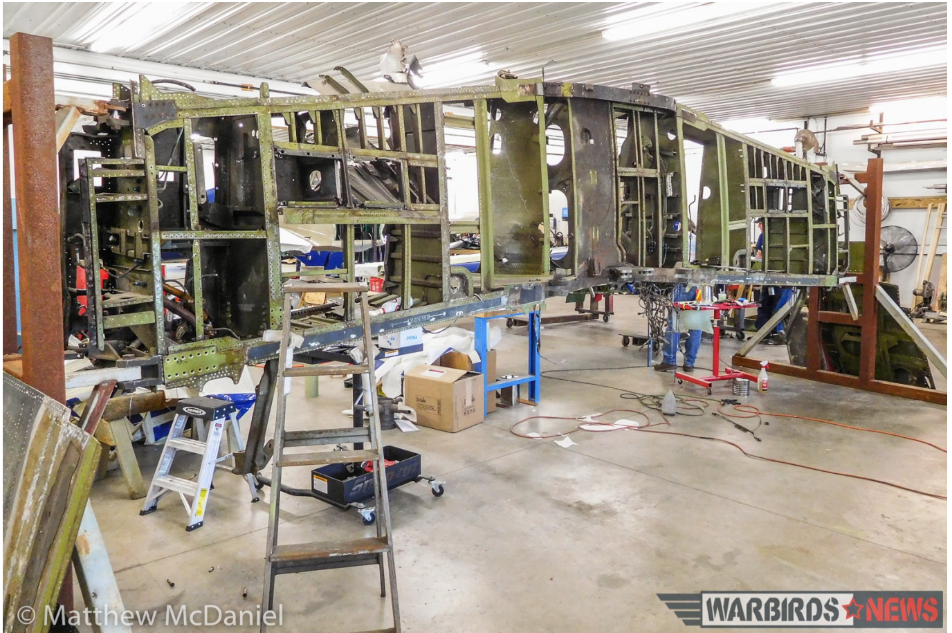
The massive center wing section of the SB2C currently resides at the back of the Tri-State shop, but it is far from a back-burner project. (photo by Matthew McDaniel)
