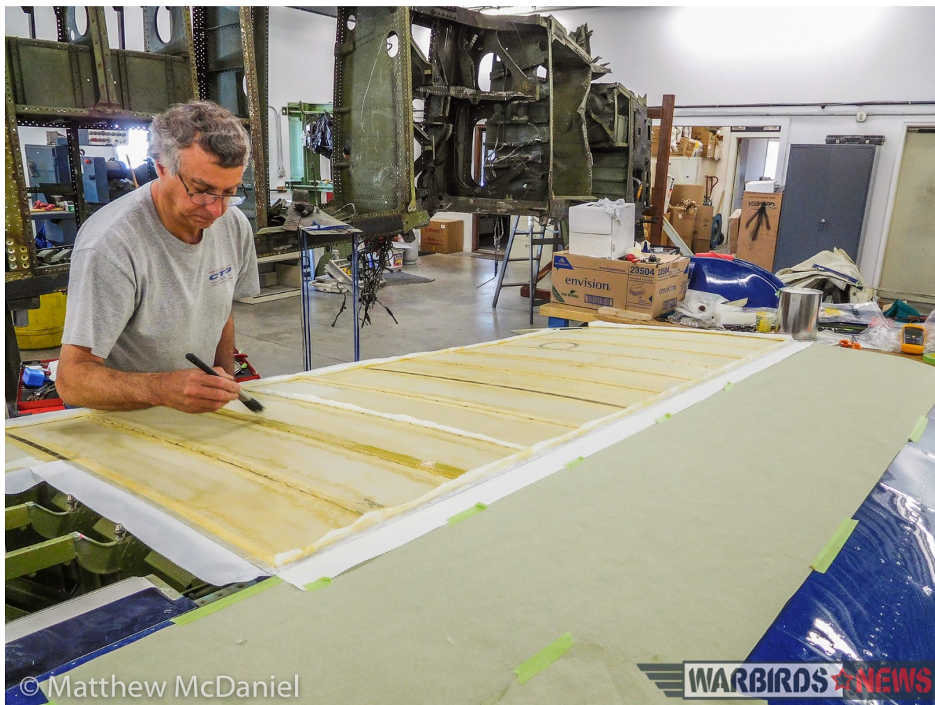
A Tri-State Aviation technician works patiently, replacing the fabric on the underside of the Corsair's outboard wing panels (photo by Matthew McDaniel)
