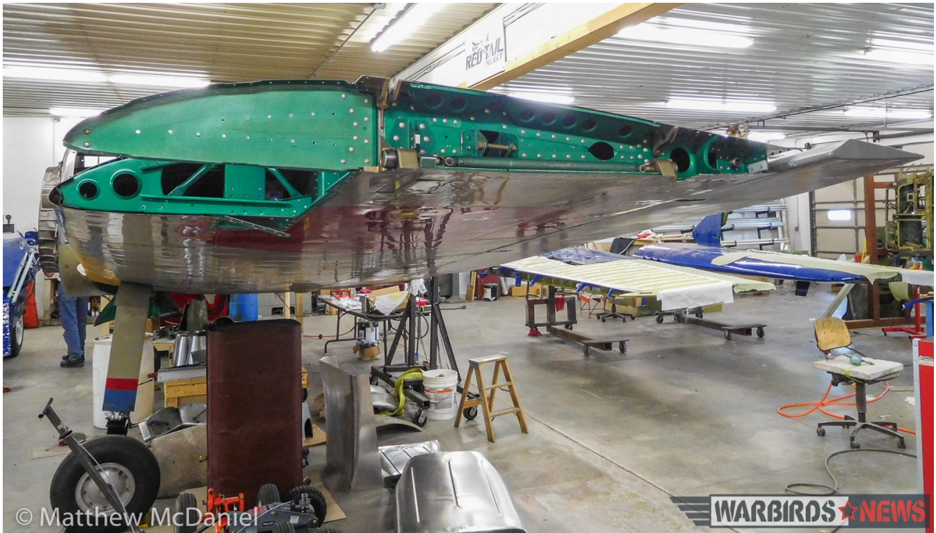
The left wing of the Flying Legends Zero, minus the foldable tip. This is one of the areas damaged in the ground accident that is being repaired at Tri-State (photo by Matthew McDaniel)
